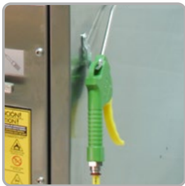
Blowgun for drying the gun interior areas.
