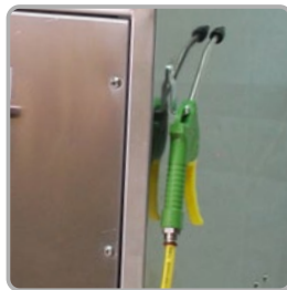
Gun with coupling to clean interior areas
