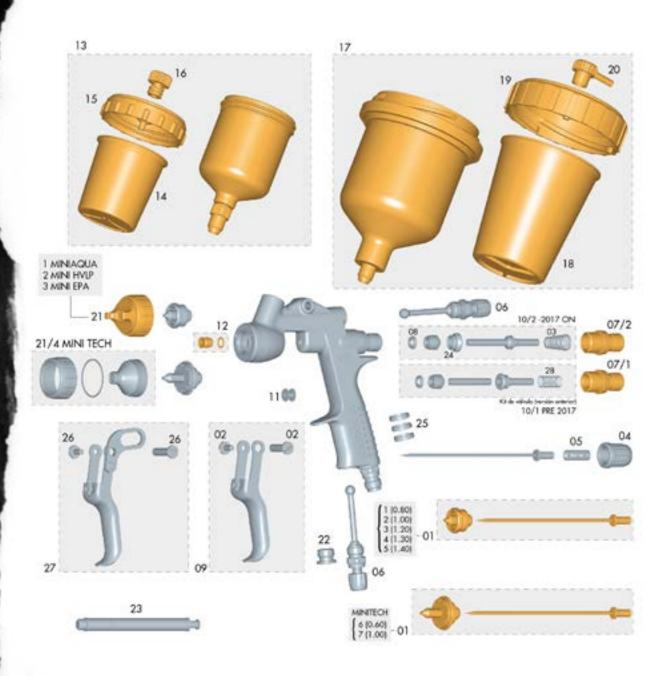
Critical parts are those that can produce a malfunction in a spray gun: Wearing parts, seals, gaskets, glands... Sagola spray guns contain **ONLY 6 CRITICAL PARTS** ( ). Just 6 references to store and provide a 100% effective after-sales service.
